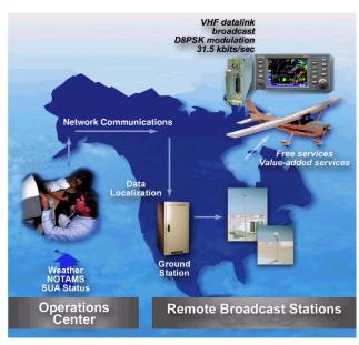
See our website at www.bendixking.com for VDL network status and coverage. Continuous coverage of most of the continental US is possible at altitudes as low as 5,000 ft. AGL, except for regions of precipitous terrain. As with all VHF communications, the line-of-sight range increases with altitude. However, there is no appreciable increase in coverage above 17,500 ft MSL. The following illustration shows how altitude influences FIS VDL coverage.
