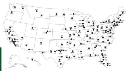
Figure 3-11 - TIS Capable Mode S Radar Sensor Sites
