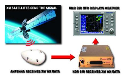
The XM Satellite Radio weather system provides continuous coverage down to ground level over the entire continental United States. A good view of the southern horizon must be available in order to receive at least one of the two satellites.
