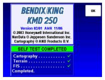
One of the following Instrument Panel Self Test Pages will be displayed depending on whether the unit is equipped with an internal GPS or is the non-GPS version.
